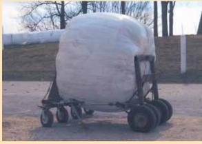
Front section rides on caster wheels and is equipped with a chain to pull the bale. Back section is equipped hinged metal "flapper brake".
