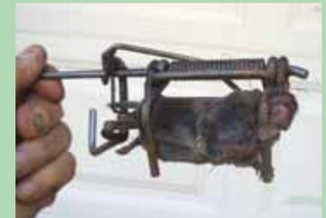
Mole trap legs clamp in and down from above (left), ensuring moles coming from either direction in tunnel will trip the trap.
