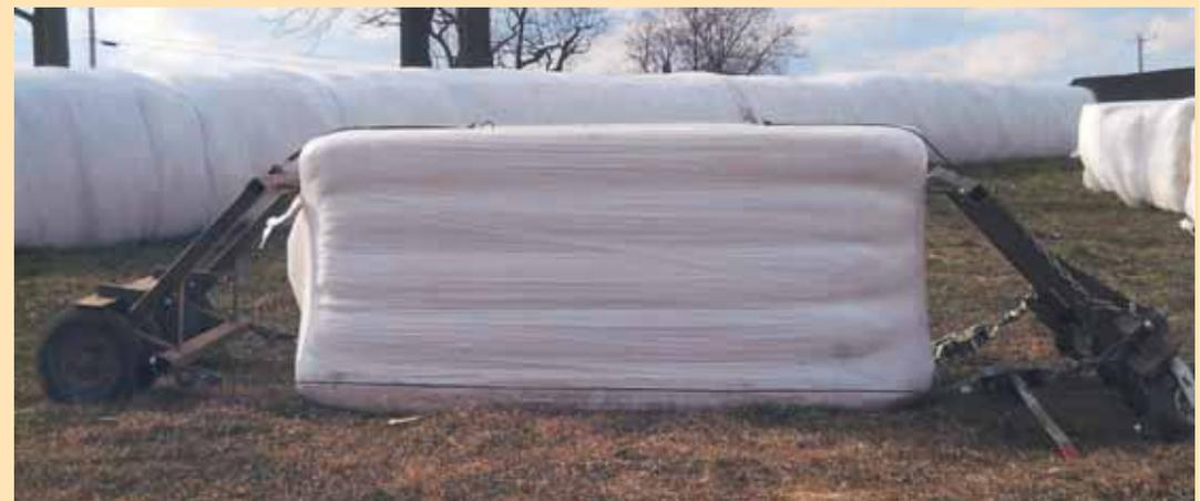
Both sections are fitted with 3-in. prongs and come-alongs that are used to crank the sections together. The prongs dig into bale and lift it off the ground.
