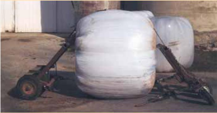
One-of-a-kind carrier lets Jesse Fisher haul a round or big square bale on 8 wheels without a tractor. It consists of 2 different sections, one on either side of bale.
