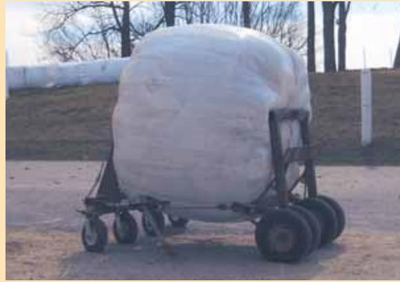
Front section rides on caster wheels and is equipped with a chain to pull the bale. Back section is equipped with a hinged metal "flapper brake".
