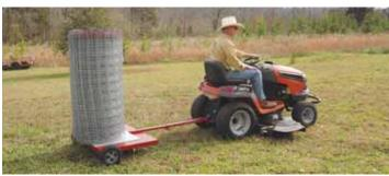
2-wheeled "fencing trailer" consists of a metal platform with a 34-in. long pole on top and a poly foot plate for the wire roll to turn on.
