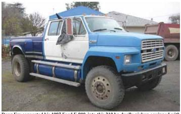
Doug Fry converted his 1987 Ford F-800 into this 210 hp dually pickup equipped with a crew cab. It's fitted with twin 115-gal. fuel tanks.
