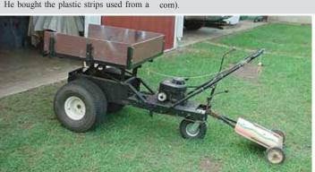
Ron Forster's home-built self-propelled cart is powered by a 3 hp engine and 5-speed transmission. The operator stands on a 2-wheeled plywood platform.
