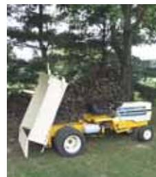
Bed lifts and lowers with an electric-powered hydraulic pump and cylinder.
