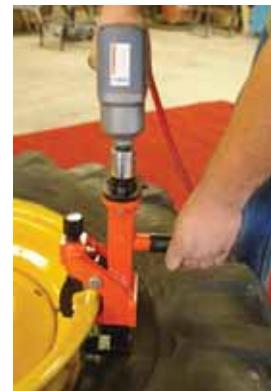
All you need to operate impact bead breaker is a 1/2-in. drive impact wrench. Handle on back of tool is used to apply leverage as you draw tire in.
