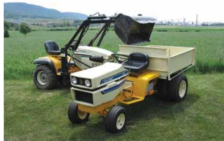
Calvin and Doug Kiffer converted a garden tractor into this "dump tractor", building the bed to match the loader bucket on their Cub 1782 tractor.
