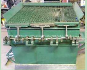
Cranks at end of machine raise and lower sections of serrated teeth that move between flat steel bars. You can see a video of it in action at the company's website.
