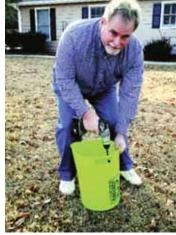
Collector tube extends up from bottom of bucket. To collect soil sample, the operator runs a cordless drill-powered auger through tube and into the ground.
