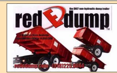
Operator sets the trailer brakes and then backs up. As the upper frame and trailer box slides back past the end of the lower frame, it dumps. No Hydraulics? Dump Trailer
