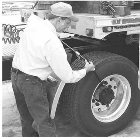
**Tire Bee repair kit uses a self-vulcanizing plug and a tool that uses compound leverage to push plug all the way through the tire. One end of tool is secured on wheel rim.**
