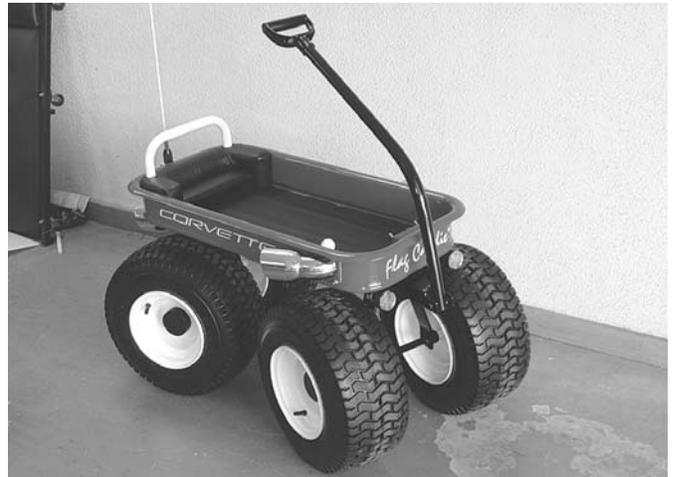
Radio Flyer wagon rides on big garden tractor tires and has a padded vinyl seat and rollbar on back. Note side-by-side Corvette C-5 exhaust mufflers.
