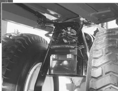
Underside of wagon shows articulated steering system.
