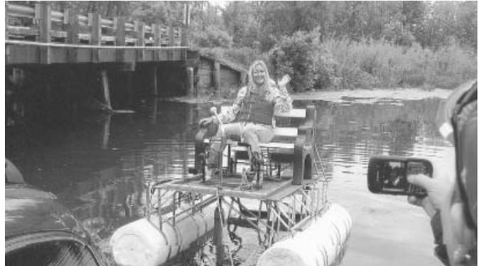
Home-built pedal boat floats on eight 30-gal. plastic drums, and is fitted with a wood and plastic seat set on a plywood floor.
