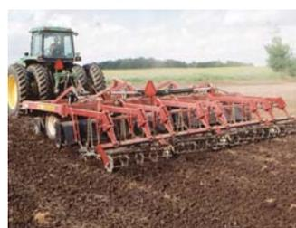
"It's equipped with ultra-shallow concave disk blades that loosen the top 2 to 3 in. of the soil, yet leave a firm seedbed that ensures accurate seed depth at planting. The leading disk blades penetrate the soil and slice residue into manageable pieces. The disk has enough weight to force the no-till coulters into the ground deep enough to allow my planter to work at optimum depth."
