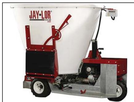
Jaylor mini-mixer has a 50-cu. ft. capacity and comes in 4 models, including this self-propelled unit.
