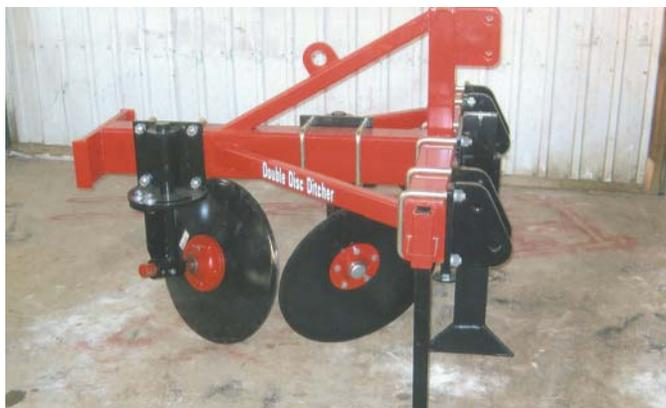
Ditcher comes with two 22-in. disc blades. Blade angle can be adjusted independently to easily vary width of furrow.
