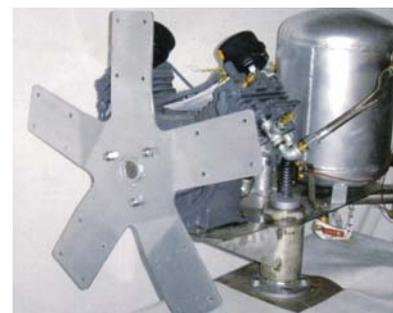
Win-Pressor turbines are designed to produce compressed air instead of creating electricity.
