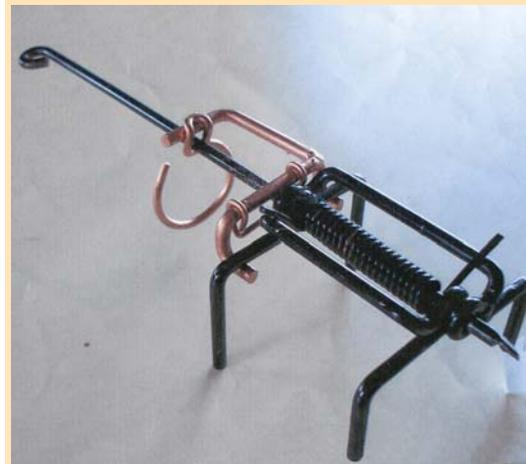
The trip mechanism on this gopher trap hangs from the tunnel roof, with trap arms to its sides.
