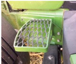
Bolt-on step kit for Deere 7000 and 8000 series tractors has a see-through design for better visibility.
