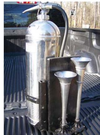
To scare away birds, Bill Jones made this loud air horn out of a 2 1/2-gal. fire extinguisher and a pair of air horns off an old fire truck.
