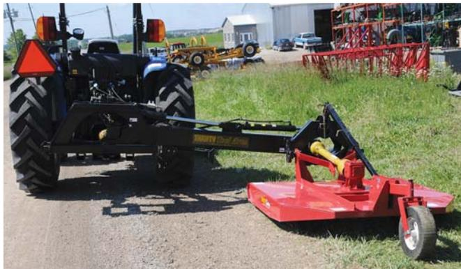
By extending or retracting a cylinder, mower can be tipped 90 degrees to cut nearly vertical bank.
