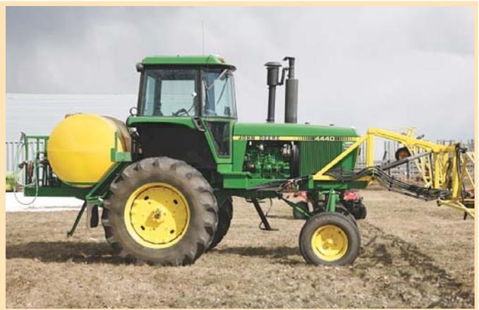
The 67-ft. boom is a 3-piece design that automatically folds back around the tractor, with 5-ft. breakaway tips at either end.
