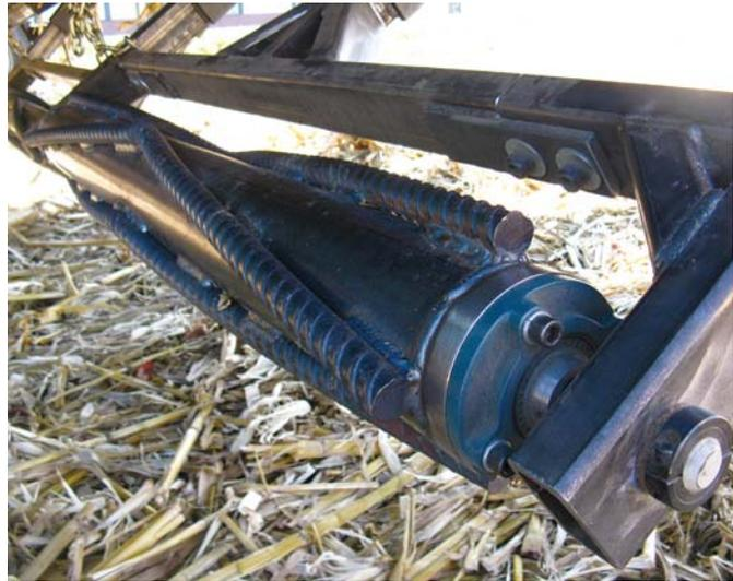
Spring tension presses stalks down and crushes them. Wrap-around rebar cleaning enhances ground action of roller.
