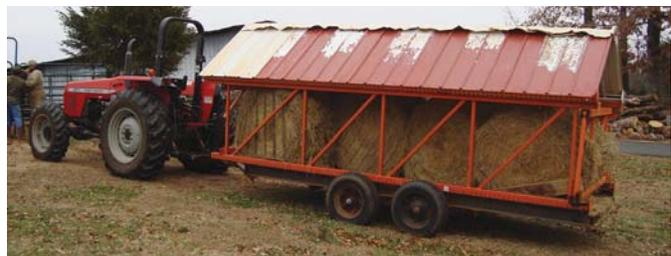
Mike Wilson made this 16-ft. long feeder using industrial warehouse shelving racks, tin off an old barn, and an old trailer. It can hold up to 5 round bales at a time.
