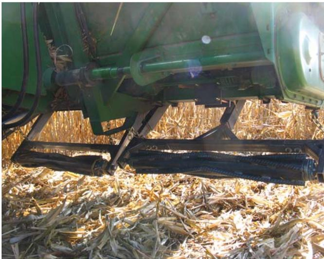
Kitchel stalk roller is designed to reduce stubble wear on tires and other equipment. Multiple 44-in. long sections each crush 2 rows of stubble.
