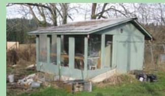
Wess Cornelius used 8 by 8-ft. plywood panels to build greenhouse’s floor, walls, peak ends and roof panel.
