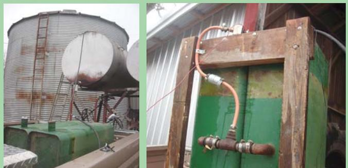
McAlister bolted together two fuel tanks off an old Oliver combine (left). He plumbed the tanks together with a T fitting and hose that goes to an electric fuel pump.
