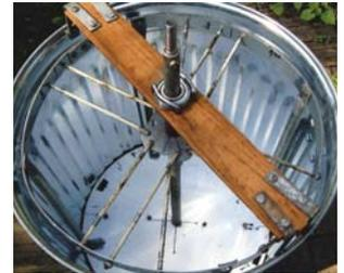
"Cage" with paired 1/4-in. dia. rods mounts inside trash can. Four honeycomb frames fit inside the paired rods.
