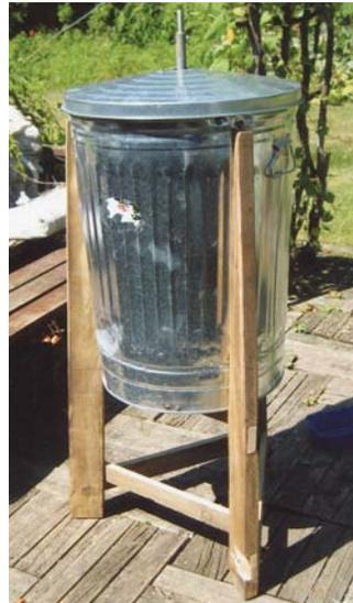
Home-built honey extractor fits inside a 31-gal. trash can that mounts on a 3-legged wooden stand.
