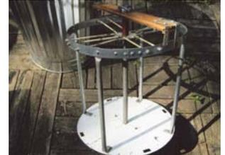
A 1/2-in. variable speed, drill is used to rotate the cage. Centrifugal force moves the honey out toward the sides of can.
