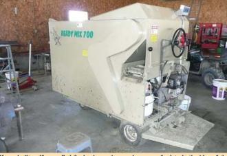
Home-built, self-propelled feed mixer mixes and conveys feed to both sides of the machine.
