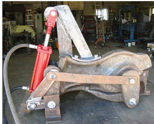
**Roger Gutschmidt converted this 100-year-old mechanical shears to hydraulic power. He uses it to cut junk steel into pieces he can sell as "prepared" scrap iron.**
