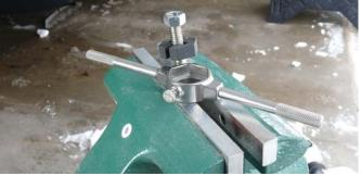
Thread Chaser tool comes with a hinged die that wraps around the damaged bolt. A T-bar handle is used to quickly restore the threads.
