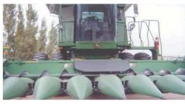
Grain Saver lays feeder house to prevent corn ears from bouncing out.
