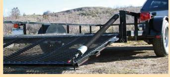
Simple spring unit takes the work out of lifting and closing heavy end gates on trailers.
