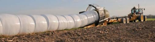
BaleLiner consists of a wrapper that piggybacks on a bale wagon for transit. Once the wrapper is unloaded, the wagon can pick up and haul up to 8 bales at a time and wrap them in the fields.
