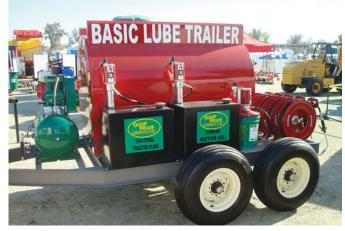
Basic Lube Cart has a 550-gal. double-wall fuel tank, a 40-gal. clean oil tank, a 40-gal. spent oil tank, a 5-gal. grease pail with a pump, and a 5 1/2 hp air compressor.
