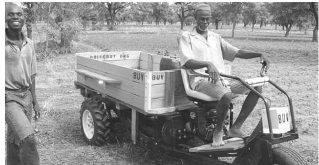
The Basic Utility Vehicle, or BUV, is a low-cost ATV without all the bells and whistles. It can be fitted with tractor-style tires for farming and logging.
