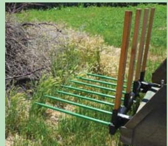
Top part of frame has 4 stake pockets to hold 2 by 4’s that form a “backstop” when hauling brush.
