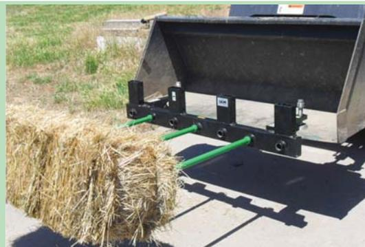
“Ultra fork” clamps onto loader bucket and comes with 7 replaceable, 32-in. long spears. Spears extend through holes in frame and are secured by lynch pins.
