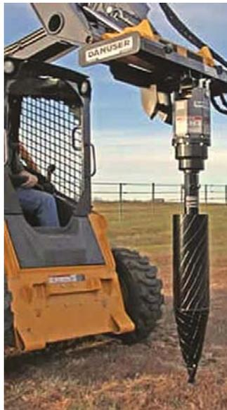
Offset cone makes auger wobble as it pushes into the ground. The result is a hole with no loose dirt in the bottom or around the top of the hole.
