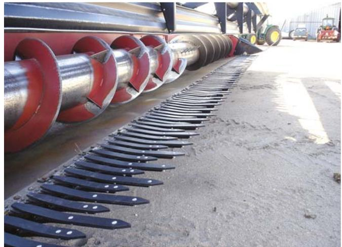
“Fingers” reach out into the crop, separating and guiding stalks into the cutterbar. Staggered positioning of 13 and 17-in. fingers enhances crop flow.
