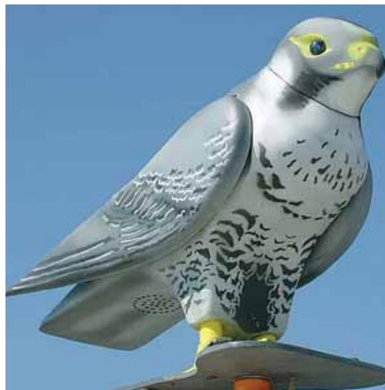
Battery-powered, robotic peregrine falcon moves its head and flaps its wings in random movements like a real bird.
