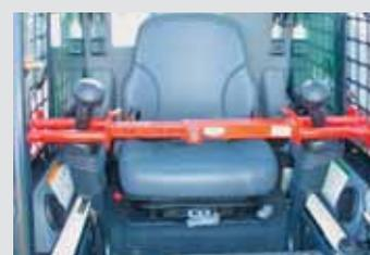
Locking device hooks over both drive controls on skid loader.
