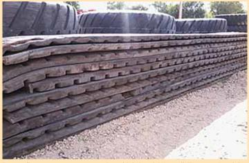
Damon Carson puts customers together with industrial "waste". For example, mining equipment tires can be cut and laid flat for use as livestock walkways.
