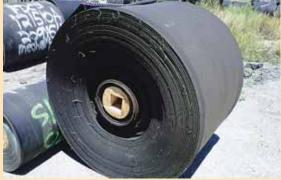
Rolls of heavy duty 4-ft. wide, 3/8-in. thick rubber conveyor belt work great for building windbreaks around livestock
