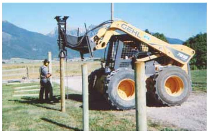
Floyd Yoder converted a hydraulic-operated, jack hammer-type concrete breaker into this skid loader-mounted post pounder.
