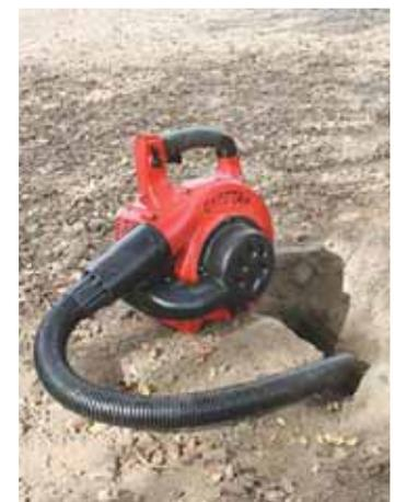
Gas-powered Cheetah uses a small engine and fan to push exhaust fumes into pest tunnels.
