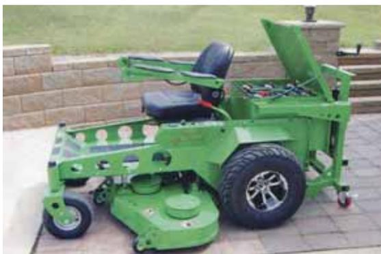
Zero turn mower uses a deep-cycle battery pack that provides an average 90 to 120 min. of mowing time. A replacement battery pack can be installed in 5 min. or less.
