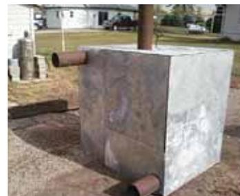
A 22-in. dia. door is cut into one end of stove for loading wood. A heat duct and cold air return are on back.
