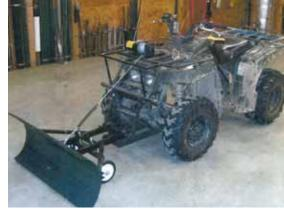
clearing a gravel driveway the wheels allow the unit to ride up slightly without catching on rocks," sourcleff.
