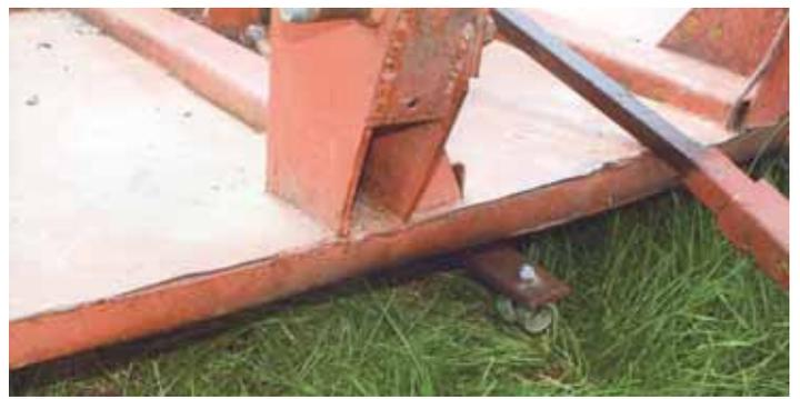
As seed falls through hole in deck, spring-loaded tines bolted to mower's flail arms work it into the ground.
