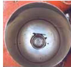
When mower is operating, the vibration is enough to shake seed through sieve of bottom of mini hopper.
