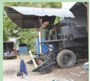
Combine's reel was moved forward to make room for a stage over the feederhouse. Corrugated steel roof extends over stage.
