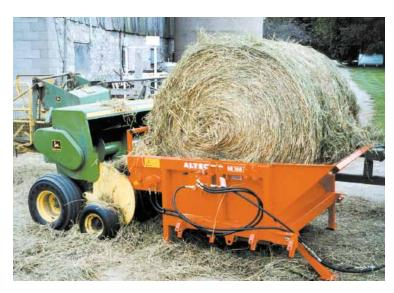
when you're done using the unwinder to make small square bales, you can remove the legs and use it as a normal bale unwinder to deliver feed into bunks or onto pasture ground."
