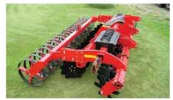
Joker compact disc combines speed with shallow tillage. It has 18-in. dia. notched blades on front and a RollFlex system at rear that smoothes the surface.
