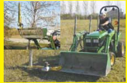
Hydraulic-powered cutter attaches to loader bucket.
