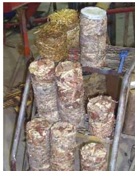
Large-scale pelletizer presses switchgrass or corn stalks into 6-in. dia. “pellets”.
