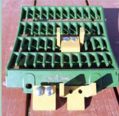
Disrupter lugs bolt to grates, left. The lugs break up crop material in corn and beans. The new concave, right, has 7/16-in. square keys instead of round bars, with 1 1/2 in. spacing between them.
