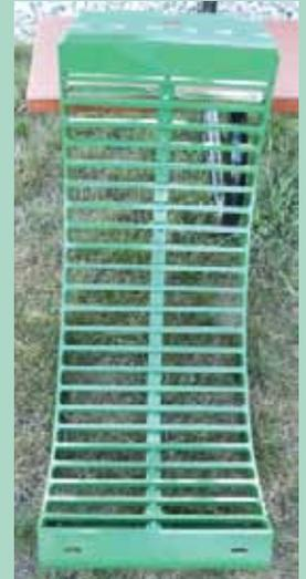
bar concave in the Deere STS rotor is that there isn't enough space between the round bars to let grain out," says Estes. "We have designed a new grate that has 7/16-in. square keys installed instead of the round bars, with a 1 1/2-in. space between them for 68 percent greater openings."
