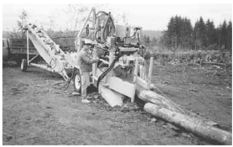
A winch pulls log into chomper. Shear blade cuts 80% of the way through log and then drags log forward, pushing the end against a fixed set of splitting blades. Once the log is split, the shear completes its cut.
