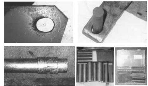
Elongated holes (top left) can be repaired by simply inserting a Repair Tech rod and welding around it (top right). Cracked bushings (lower left) can be welded right on a rod. Two kits are available (below right).
