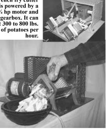
To make French fries, operator drops in one potato at a time and uses a foot pedal to activate the potato pusher.
