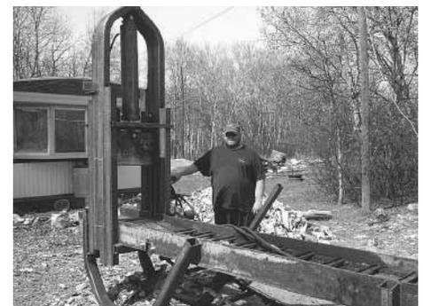
off a hydraulic pump on my truck. I set the pressure at 2,100 psi, which gives the blade about 40 tons of down pressure.”
