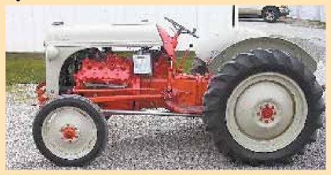
Kit costs \$1095 and contains all the hardware needed to connect the V-8 engine and clutch assembly to the Ford 8N transmission and frame. Knasel says it takes about 8 to 10 hours to install.
