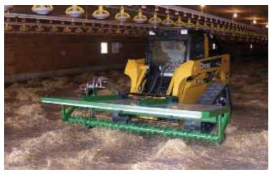
leveling, two smaller casters for support, and tines spaced an inch apart. Replacement tines are available at TSC stores.
