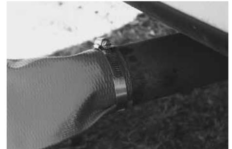
Rigid plastic adapter clamps onto vehicle's exhaust pipe.
