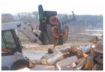
System lets operator pick up whole logs, saw them to firewood lengths and split the blocks, all without leaving the skid steer seat.
