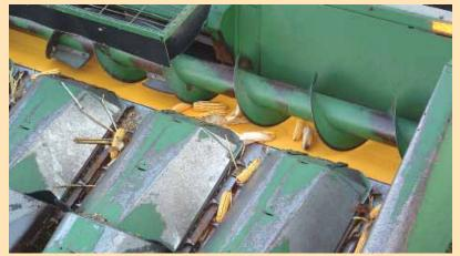
Trough liner kit does not require removal of auger for installation. It's available for Deere, Case IH, and New Holland corn heads.
