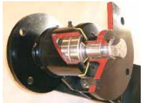
Coulter kit includes 18-in. 13-wave boron "earthenharden" coulter blades, left. Kit, right, is now fitted with 4 bearings to make it even more heavy-duty. Works in wheat stubble and corn stalks. Cuts up trash so you can plant days earlier.
