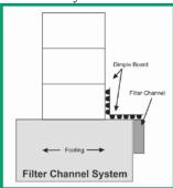
The system works well in most soils, the only exception being fine sand. If you are installing it in fine sand, or you're concerned about your soil plugging the system, just apply a minimum of 2 in. of BB shot rock (1/8 to 1/4-in.) or concrete sand around the mesh drain to prevent it from plugging. It's a lot less work than the amount of rock necessary to install a 3-in. drain tile system.
