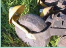
Rotating "cup scrapers" bolt onto air seeder's packer wheel mounting arm at about a 45 degree angle. Scraper is offset 1 in. from center of packer wheel.
